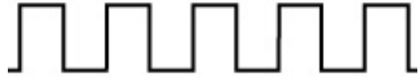
A Modulated Square Wave appears as a High/Low signal repeated rapidly over and over.
